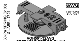
VOH501-32AVG OPERABLE BRIDGE, PLAIN HANDLE AND EMERGENCY VENT SUB-ASSEMBLY
