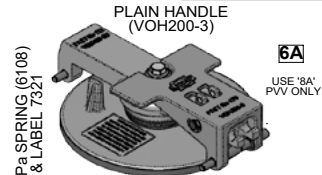
VOH501-32A OPERABLE BRIDGE, PLAIN HANDLE AND EMERGENCY VENT SUB-ASSEMBLY
