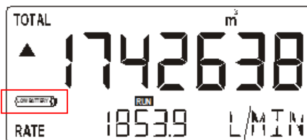
Fig. 4: Example of low-battery alarm.
